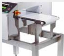
Hygienic design features include an open frame construction that prevents build up and facilitates fast and easy clean-up and sanitation.
