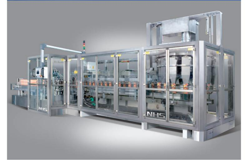
For automatic, **direct fill of powders, granular products** and random packaging of small/medium size items directly **into cardboard cartons**. The Senzani flagship NHS vertical cartoning machine models are the most performing units of the entire Senzani VECA category. Many lines are constantly producing in excess of **500 cartons/min.** (24 hours/day, 7 days a week).
